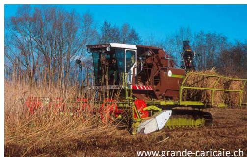
Switzerland → Elbotel, loading capacity of 23 bales, ground pressure:  $240\text{g/cm}^2$
