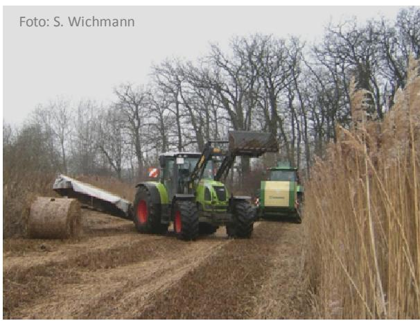
Tractor with Terra wheels, baling press with tandem axle
