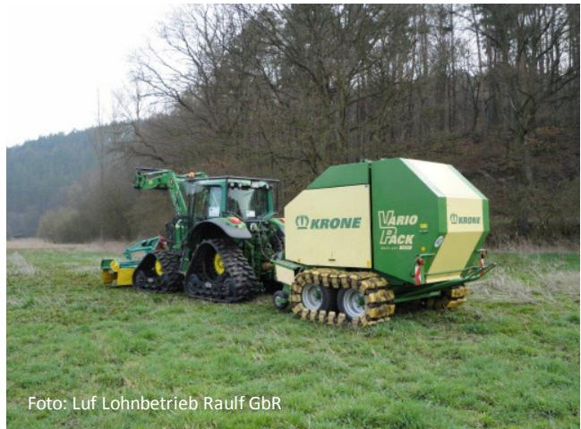
Tractor with Soucy tracks and baling press with 'tracks' ( $140\text{g/cm}^2$ )
